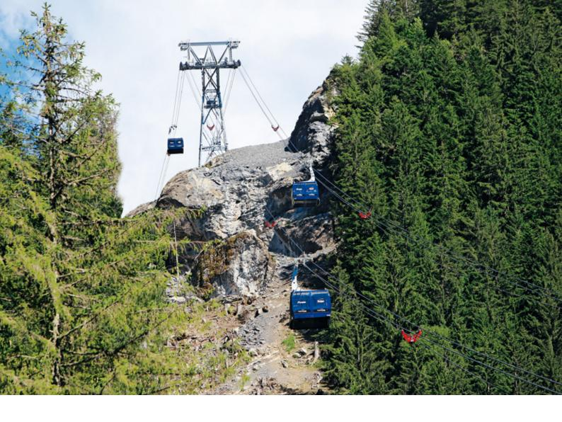
Tricable ropeways have a **single haul rope** and **two carrying ropes**. The system is implemented using detachable grips and offers very high transport capacity. They guarantee increased wind resistance and can also cross major spans of over 2,500 meters. In addition, the **3S system** is useful for bypassing obstacles in cities.
